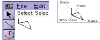
The longest of the three lines is always the x-axis, the next longest is always the y-axis and the shortest line is always the z-axis.
